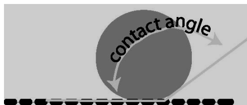
Ball "Rolling Effect" of an ultra-hydrophobic surface (over 145 deg. of contact angle)
